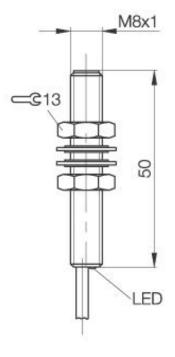
Inductive Sensors BES M08MI-PSC15B-BP03 M 8 x 50 normally-open Sn=1,5mm shielded
